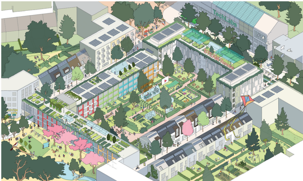
Fig.15: Multi-plot perimeter block with private back gardens and a resident-only communal garden.
